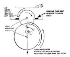
Rotate the large gear (ref. 111) to line up the holes with the U/D gears (ref. 114) mounting post. (See diagram)
