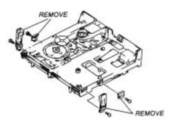
Slide the table forward to expose the gear assy. Take care not to damage or disconnect the flex cable attached to the sensor board. Remove the Rubber cushion. (see diagram below)
